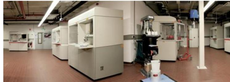
Our two large-frame laser sinter machines are part of the EOSINT range by EOS and we have one example each of the P700 and P380 range. The adaptable P380 can work with RM-06, RM-07 and RM-08 material while the P700 functions with RM-06 only. Our two laser sinter machines offer a diverse range of size options; the P700's build volume is 700 x 380 x 580mm while the P380's is 340 x 340 x 620mm. All TMG's rapid manufacturing machines are serviced regularly to ensure reliability.
